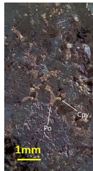
Figure 4: Field photo from 18AFAC20677 showing chalcopyrite (Cpy) and pyrrhotite (Po)
