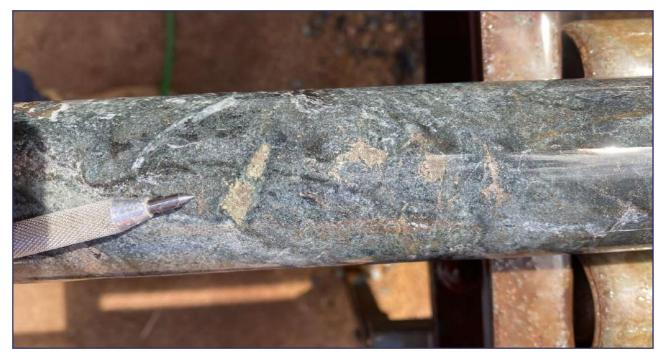
Figure 2: Two-phase sulphide blebs (pyrrhotite-chalcopyrite) in gabbro with high carbonate assimilation – Snowys Dam Formation (21AFDD116, ~619.7m)
