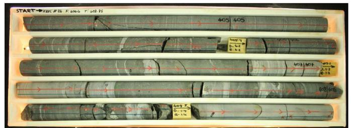
Figure 2: Diamond drill core laid out in core tray
