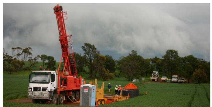
Figure 3: Diamond rig drilling on cropped land
