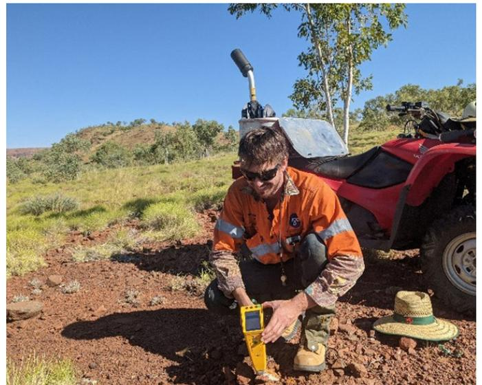
Figure 2: Geologist using pXRF to analyse a rock chip sample
