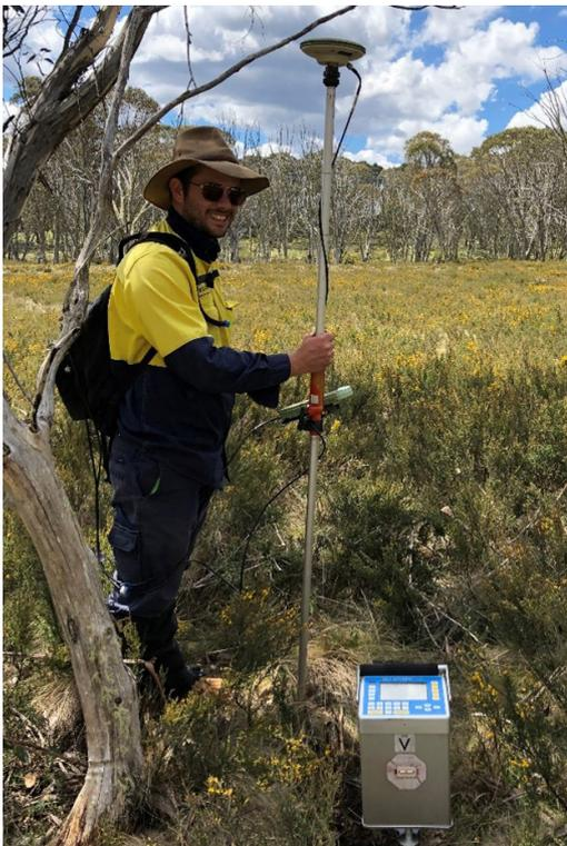
Figure 1: Example of ground gravity survey carried out on foot
