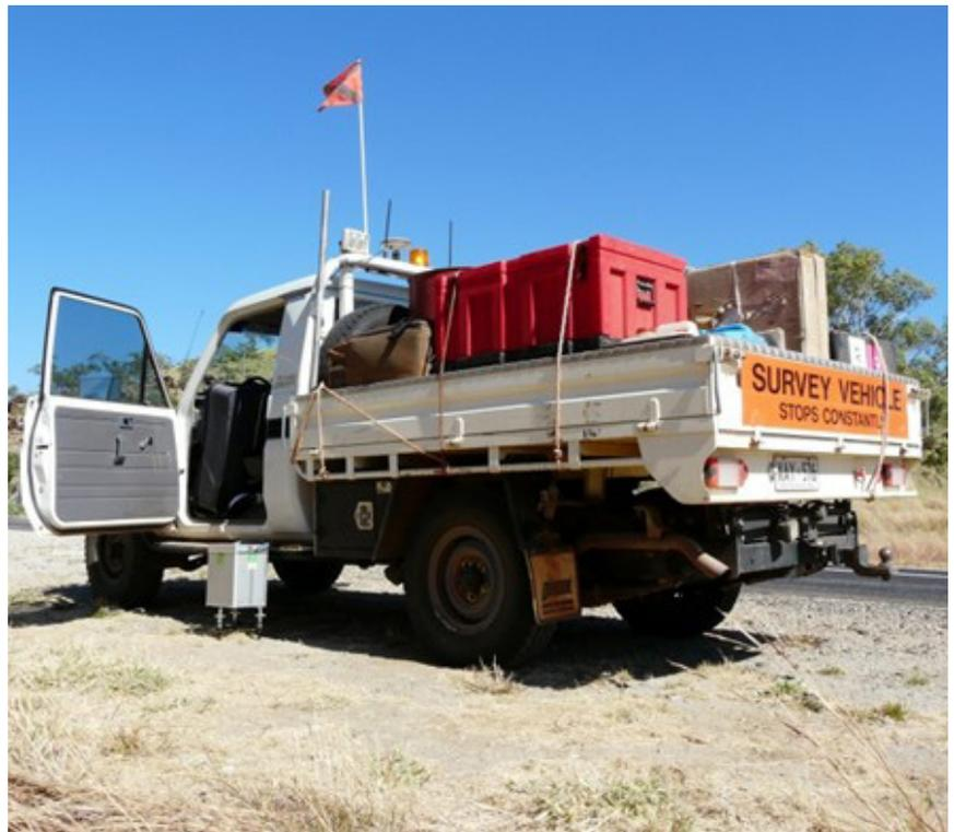
Figure 2: Roadside ground gravity survey carried out with light vehicle
