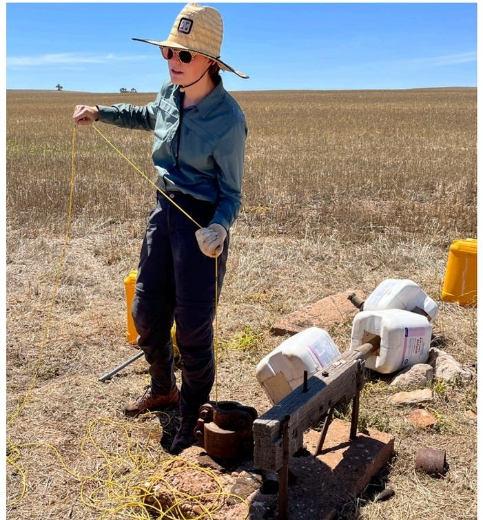
Figure 2: Using a hand bailer to collect water from a bore
