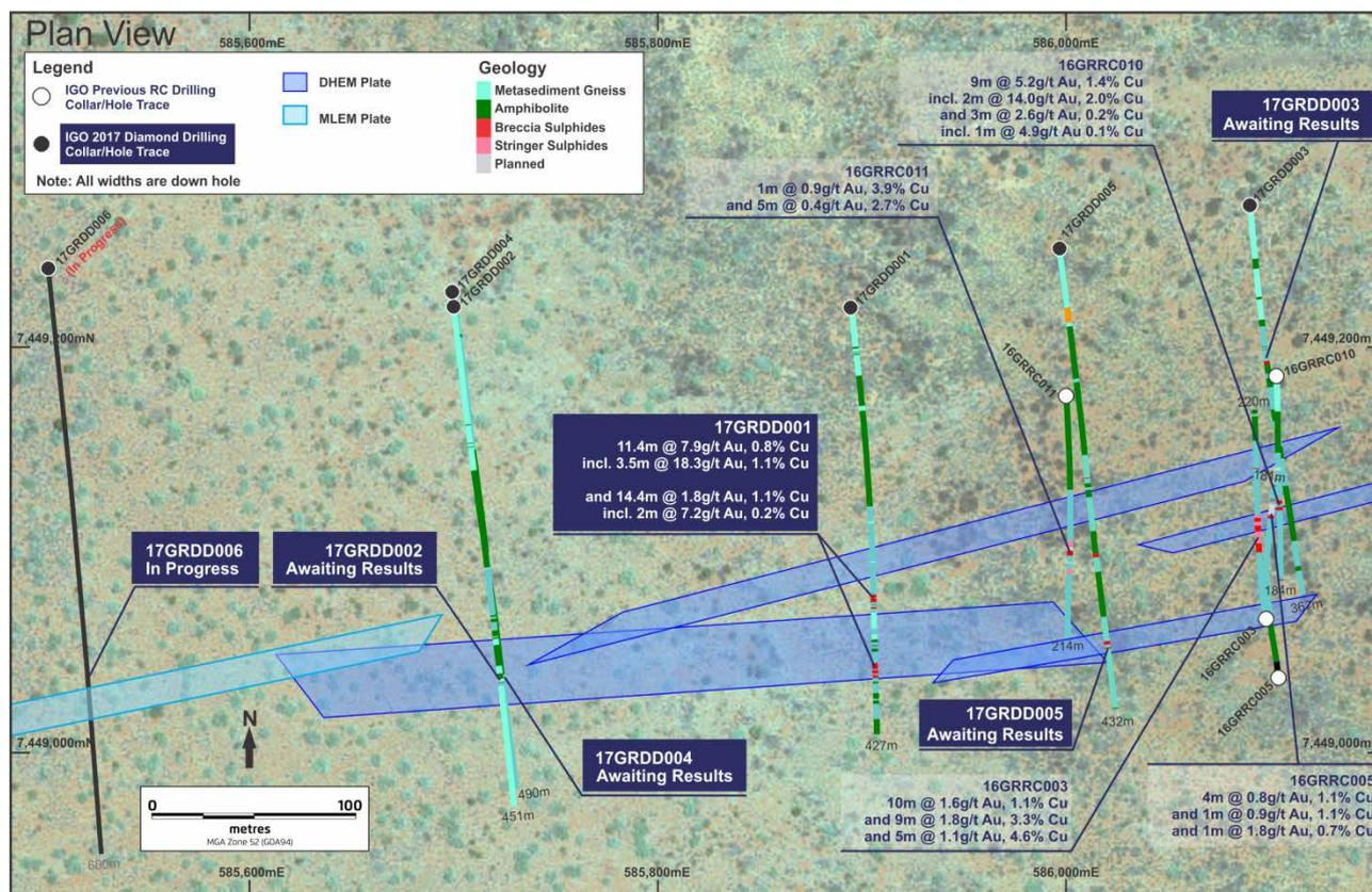
Figure 2: Plan projection of Grapple Prospect drill holes
