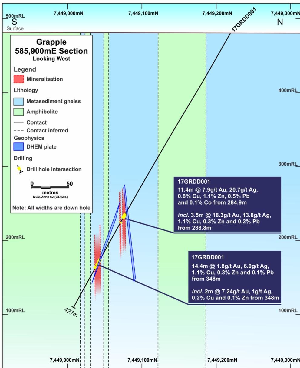
Figure 3: Simplified cross section of 17GRDD001 looking west
