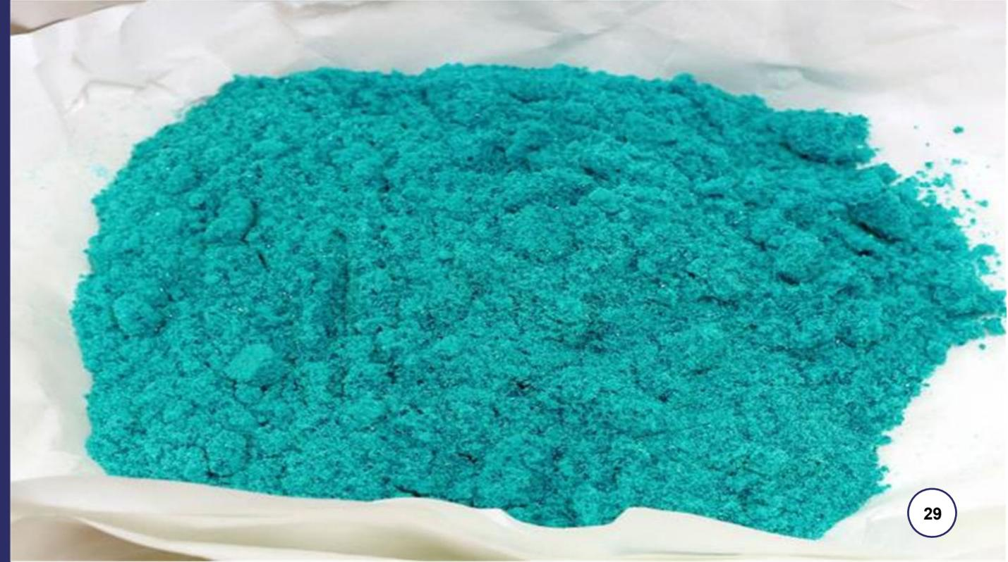
1) Photograph to the RHS is of the 1.6kg of nickel sulphate hexahydrate crystals produced in the metallurgical testwork. Photography by Karel Osten, Wood Plc
