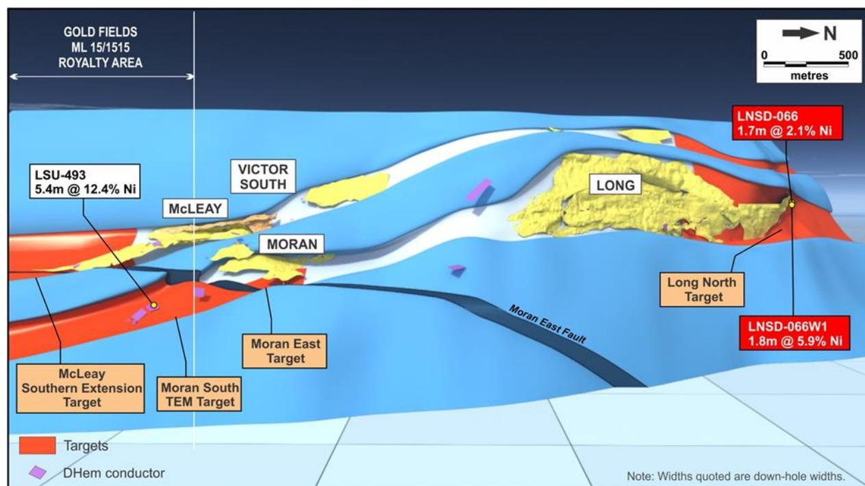
Figure 3: Long Operation – Longitudinal Projection showing Target areas, DHEM conductors and significant intercepts (>0.5% Ni)- (see ASX release dated 10 December 2014 for further detail on the Moran South drill result).
