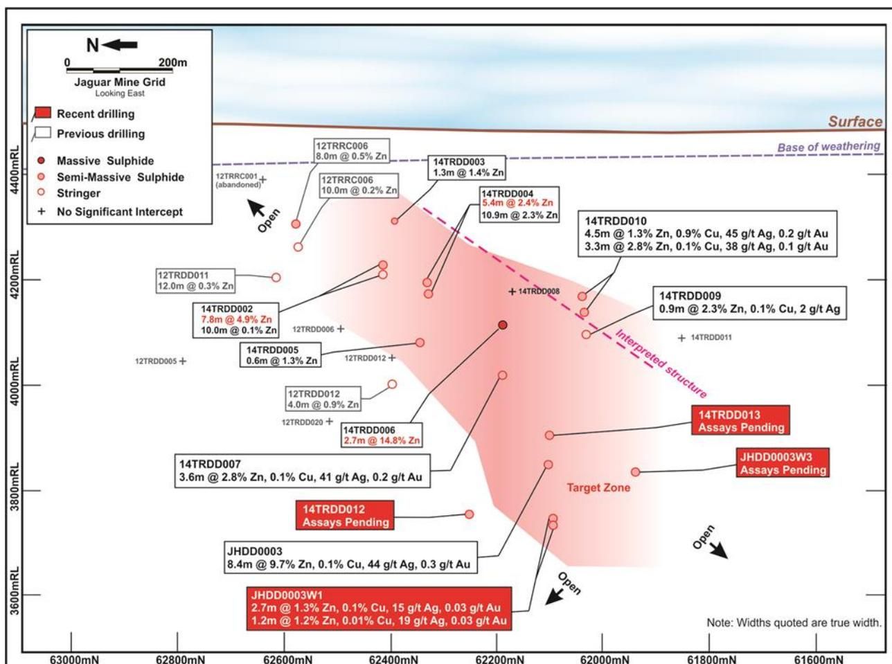
**Figure 6 : Jaguar Operation Regional Exploration - Triumph Long Section. (see ASX release dated 22 September 2014)**
