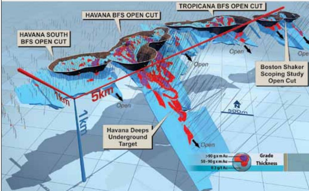
Figure 9: Tropicana JV - Proposed Boston Shaker, Tropicana, Havana and Havana South open pit outlines, g/t Au x thickness (m) contours in 3D isometric model.
