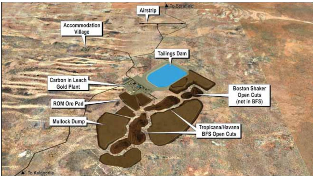
Figure 7: Tropicana JV - Computer generated model showing the layout of proposed Tropicana, Havana and Boston Shaker open cuts, mullock dumps, gold plant, tailings dam, airstrip and accommodation village.
