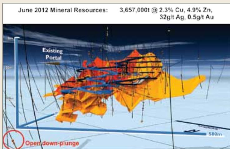
Figure 12: Stockman Cu-Zn-Ag-Au Project: Wilga Deposit - 3D isometric projection showing mineralised envelopes, drilling, planned development and down plunge mineralised intersections.
