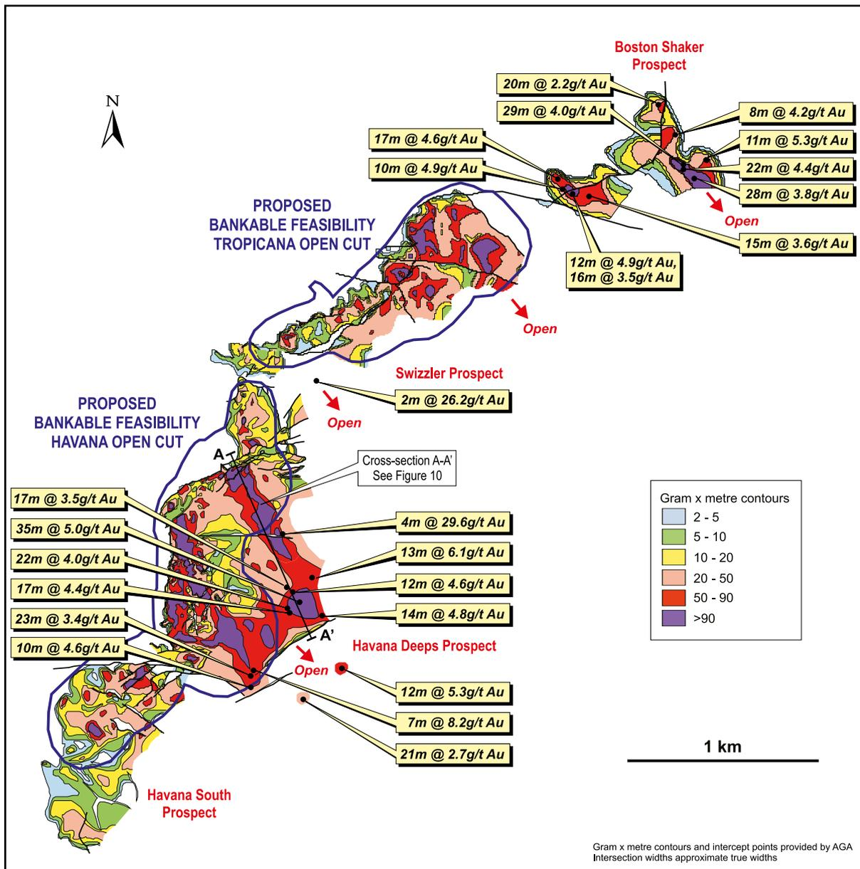
**Figure 9:** Tropicana JV – Proposed Tropicana and Havana BFS Open Pit Outlines, Prospect Locations, g/t Au x Thickness (m)
