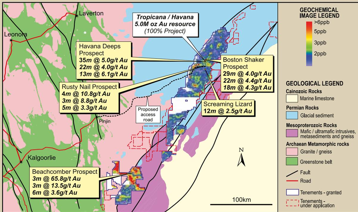
**Figure 7:** Tropicana JV – Tenure, Tropicana and Havana Resource Location, Gold Geochemical Anomalies, Significant Drill Intercepts Outside June 2009 Resources and Selected Prospect Locations
