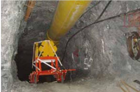
*Portable underground electromagnetic EM Torch system*
