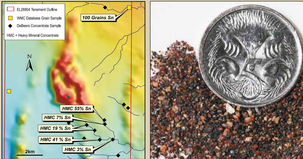
**Figure 24:** Birrindudu – (a) Tin Rich Heavy Mineral Concentrate Locations Over Aerial Magnetic Image
