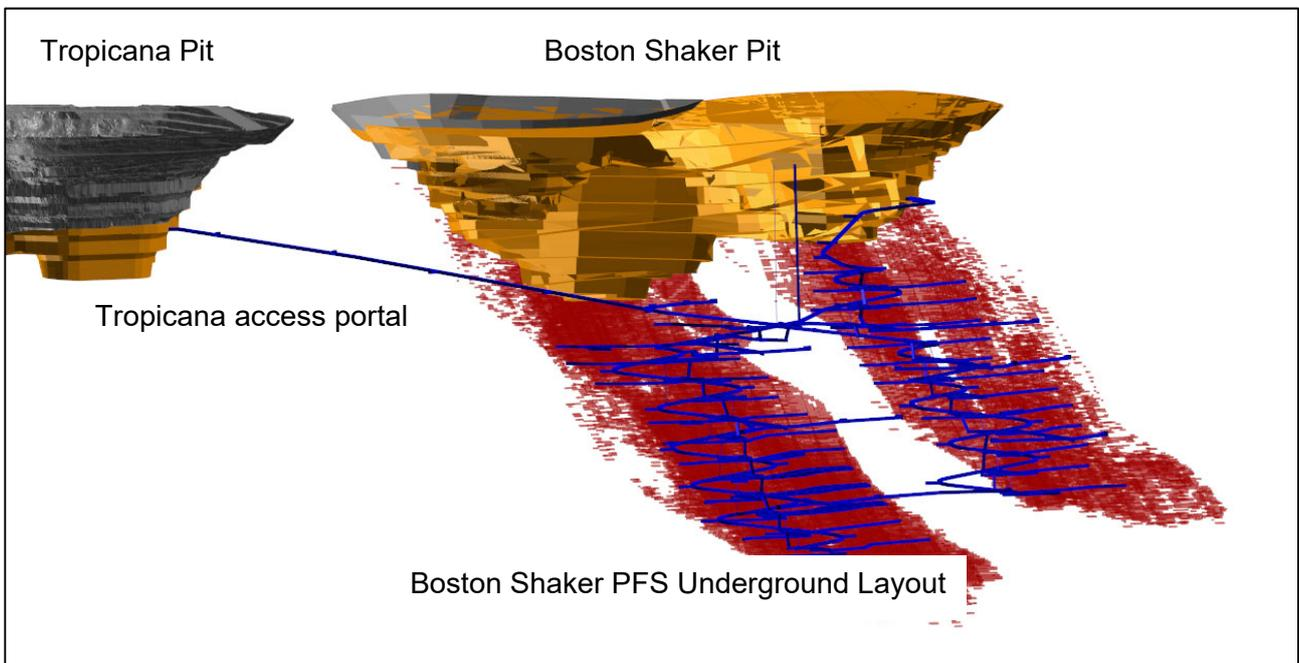
**Figure 2: Boston Shaker Open Pit, Underground Development and access link to Tropicana**
