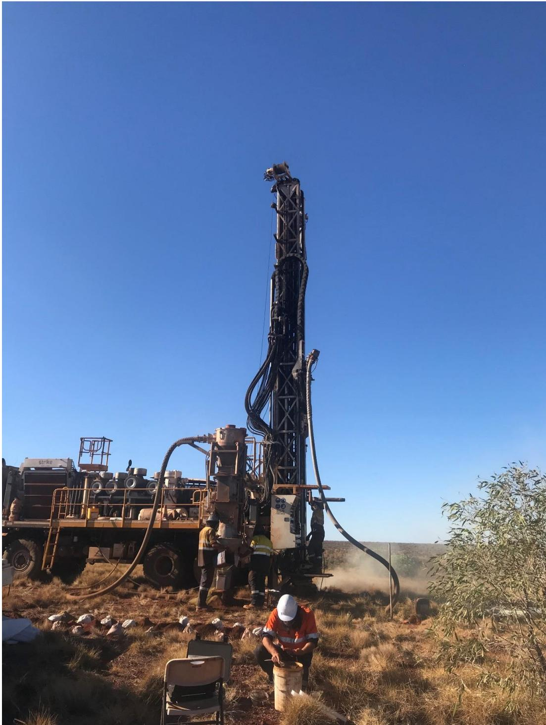
*Figure 4 - RC drilling at the Lake Mackay Project, May 2019*
