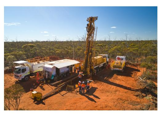
Figure 1 Diamond Drilling (DDH1 Rig) at Symons Hill
