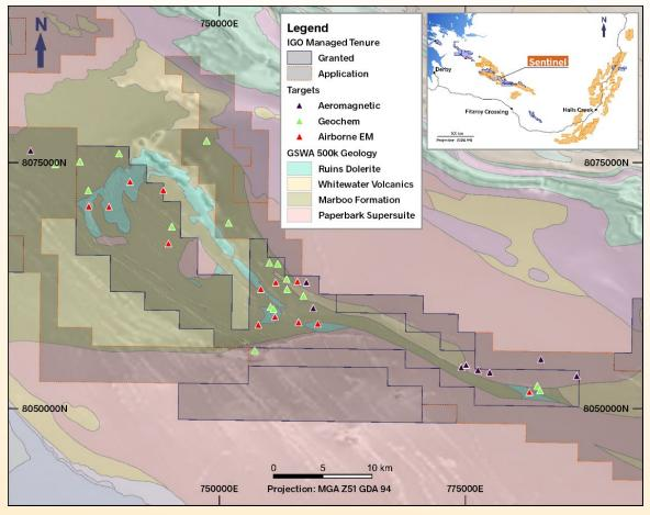
Figure 2: Sentinel area, where multiple geophysical & geochemical anomalies are the focus of ongoing ground follow-up
