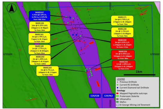
*Figure 3 – map of the Jailbreak Prospect showing the location of the latest results of the 2023 drilling.*
