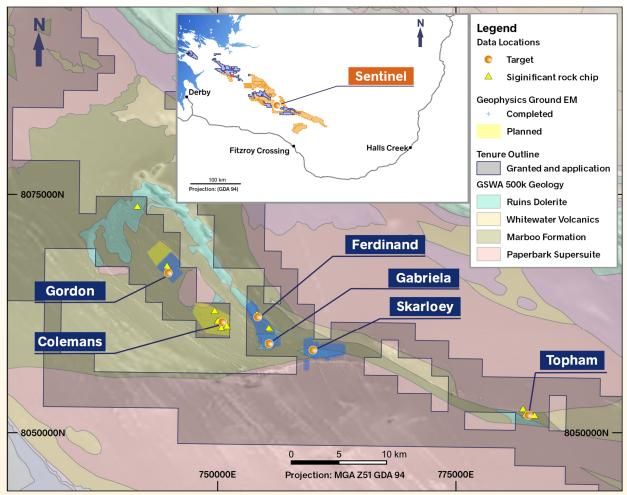
Figure 1: Map of Sentinel area showing extensive areas of planned ground EM surveying and the Skarloey prospect where limited ground EM in 2021 has defined a 9,000S conductor.
