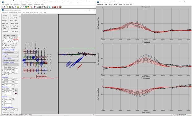
Figure 3: Left - Plan view showing all Skarloey conductors, Skarloey\_A\_v1\_9000S highlighted in red. Centre - View from the northeast showing the Skarloey\_A\_v1\_9000S conductor in red. Right - MLEM profile showing late time channel 30-35 of field data (black) and model response (red)
