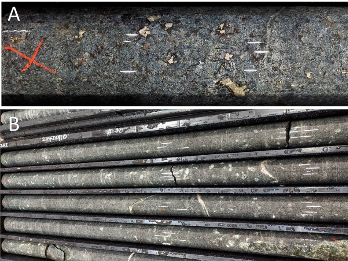
Figure 12 - Magmatic textures at the Western Eye Prospect. A) Blebby Fe-Ni-Cu sulphides in coarse-grained olivine websterite at 275m (core size HQ). B) Olivine websterite, with large, crystallised carbonate-silica vesicles at 330m (core size NQ).
