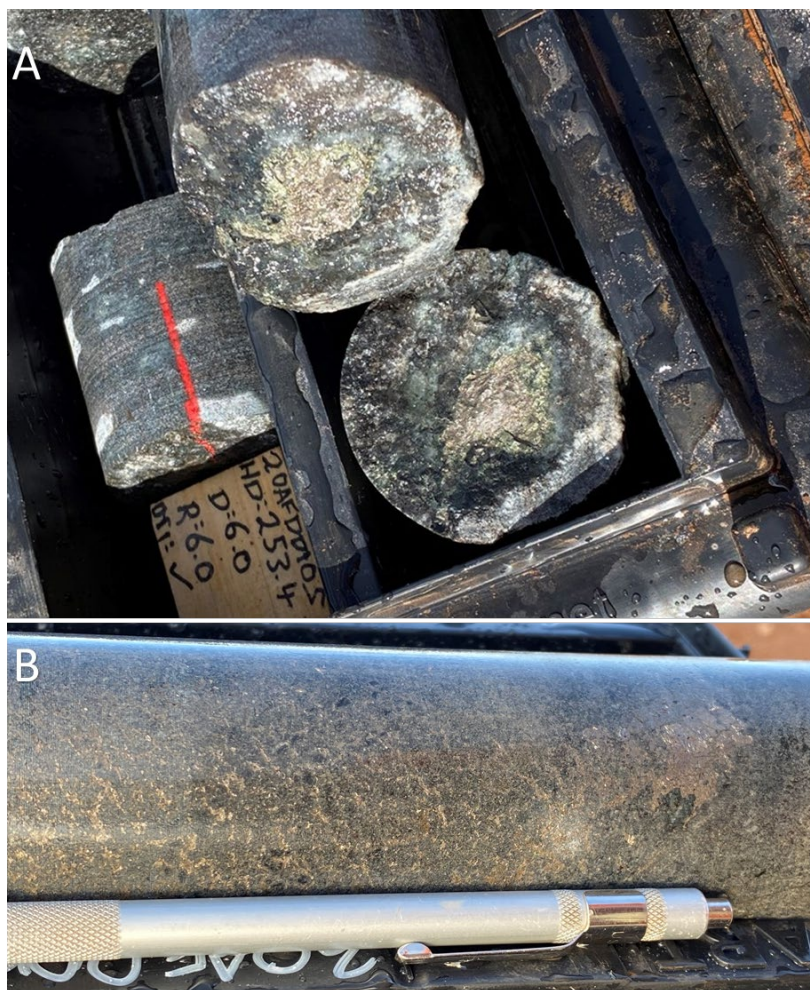
Figure 17 - Magmatic sulphide textures at the Ecliptic Prospect. A) Orthocumulate olivine gabbronorite with blebby Fe-Ni-Cu sulphides at 252m (core size HQ). B) Feldspathic Orthocumulate websterite with net-textured Fe-Ni-Cu sulphides at 276m (core size HQ).
