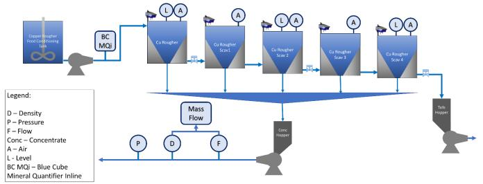
Figure 1 - Physical Layout of the Nova Copper Rougher-Scavenger Flotation Circuit at Nova.
