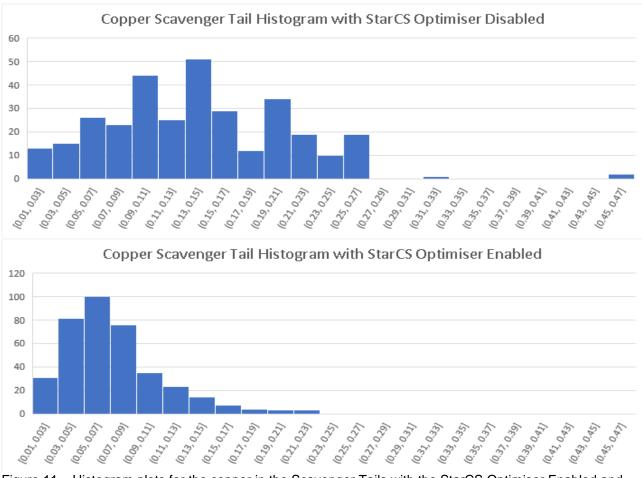
Figure 11 – Histogram plots for the copper in the Scavenger Tails with the StarCS Optimiser Enabled and Disabled
