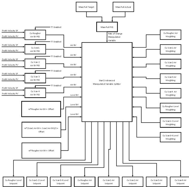
Figure 8 - Block diagram showing the main inputs and outputs required for the StarCS Optimiser.
