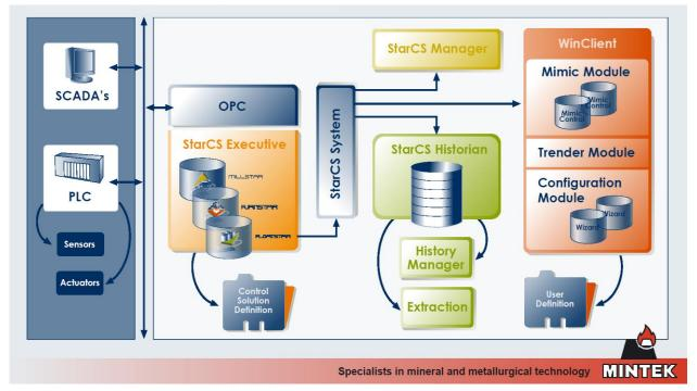
Figure 3 - StarCS modular software configuration.
