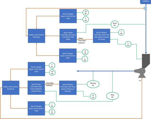
Figure 5 - Control strategy implemented on CRSC Hopper
