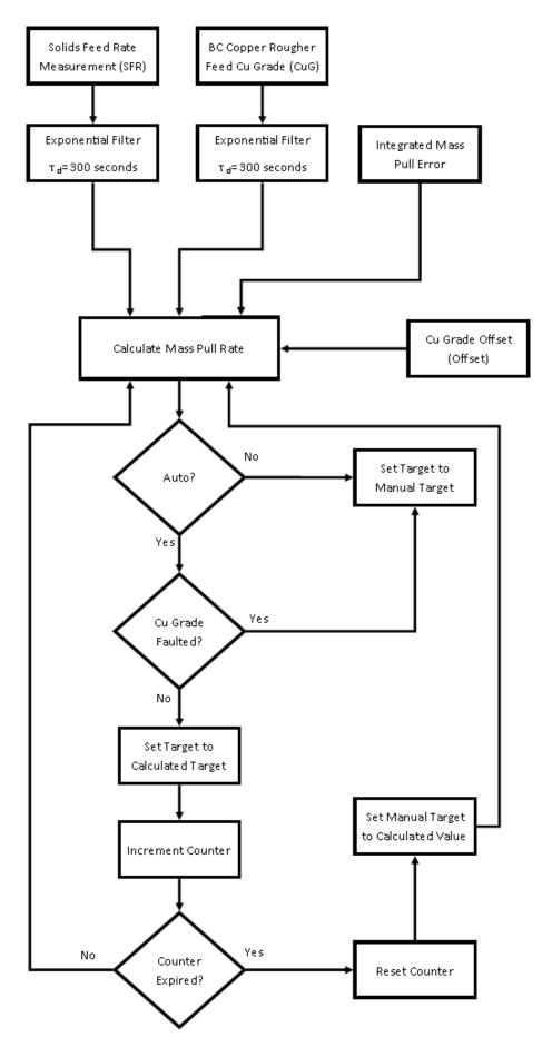
Figure 6 - Logic Diagram for calculation of Mass Pull Target.
