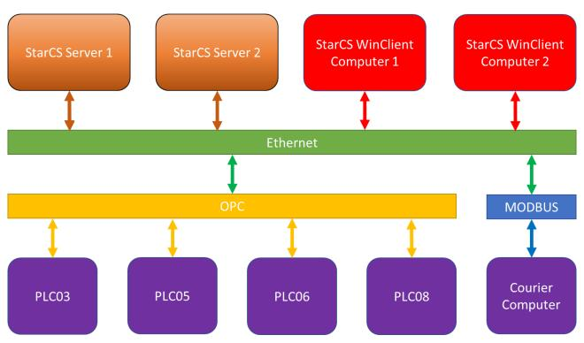
Figure 2 - Hierarchy of physical installation of StarCS at Nova.
