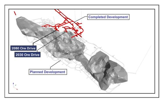
Figure 3: Status of current development showing location of 2030 and 2080 ore drives
