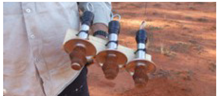
Figure 2: Close-up of magnetic lag sample attracted to plunger magnets. When the ring is at the top of the plunger, the magnet is pulled and sample is released
