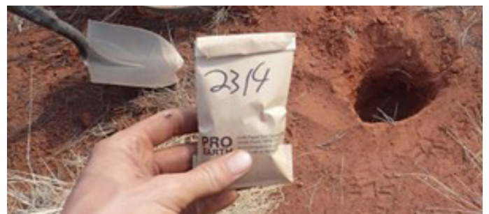
Figure 4: Example of hand auger sample site with sieve and shovel in background and sample packet in foreground
