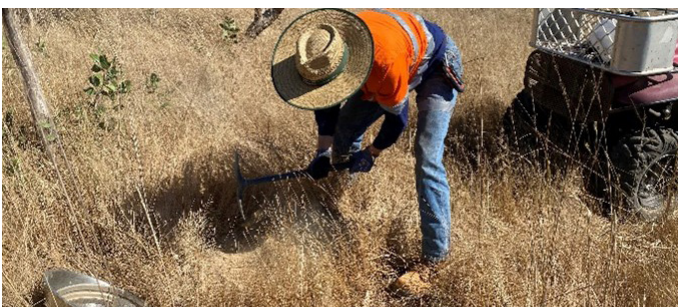
Figure 3: Pick being used to excavate soil sample with scoop, sieve and receiving pan in foreground
