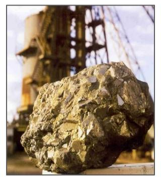
Nickel sulphides are very conductive and can be detected using electromagnetic geophysicial technology
