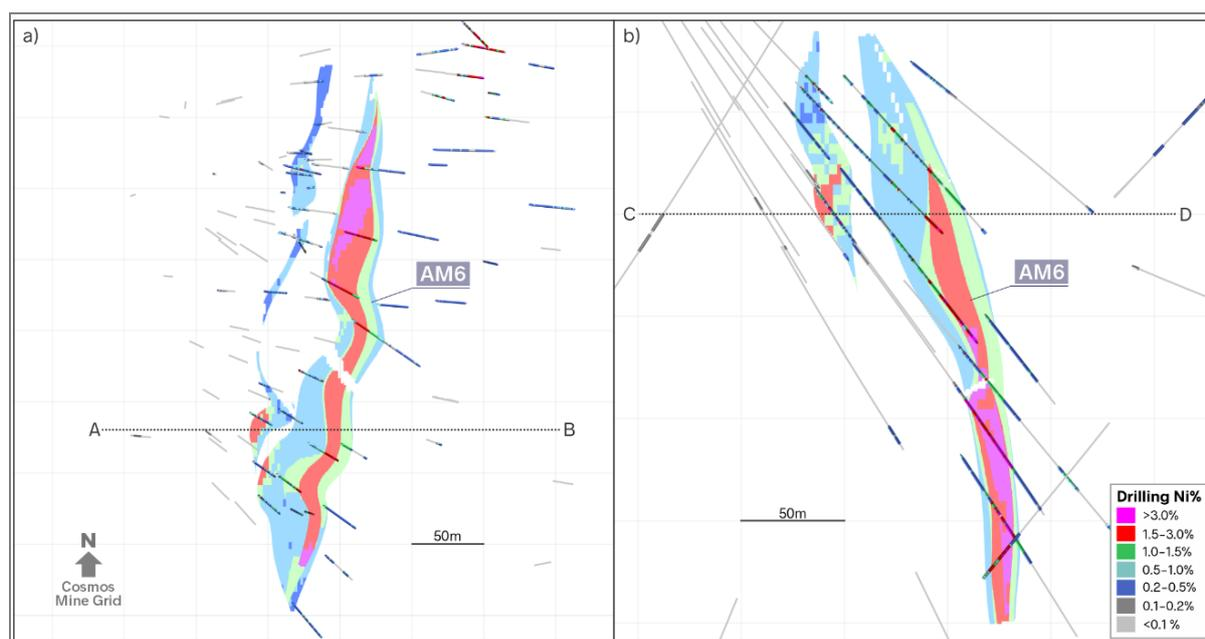
a) Plan view at level C to D denoted by the dotted line in the image to the right. b) Section view at northing A to B denoted by the dotted line in the image to the left.
