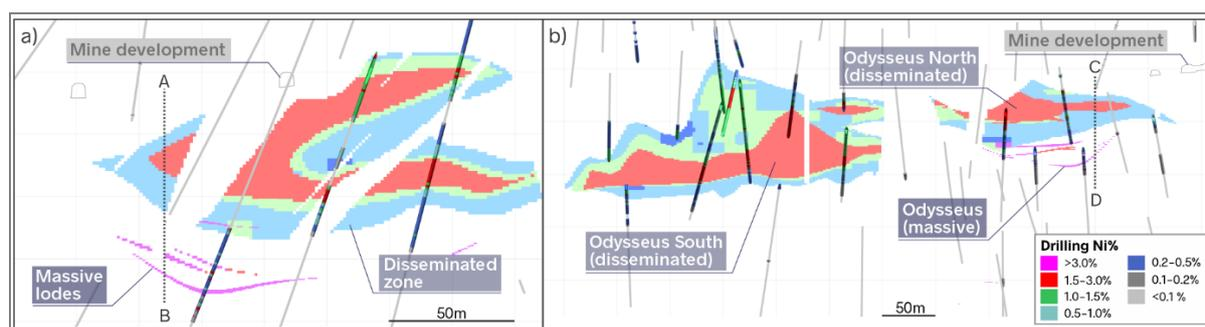
Notes: a) Section looking east through ODN's MRE model on section line C to D denoted by the dotted line in the image to the right. b) Long section looking north through ODN and ODS on the section line A to B denoted by the dotted line on the image to the left.
