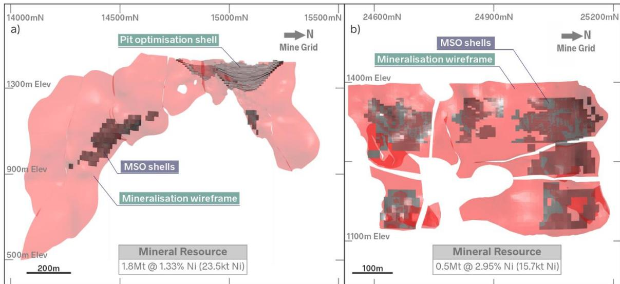
Notes: a) Long section of the Diggers Deposit looking west. The Diggers mineralisation wireframe depicted in pink represent the limits of modelled mineralisation. The Diggers pit optimisation shell and MSO shape depicted limit the MRE reporting using RP3E constraint. b) Long section of the NMDB deposit showing the mineralisation limits and MSO shells that represent the FY23 MRE. Only fresh mineralisation is reported in both estimates.
