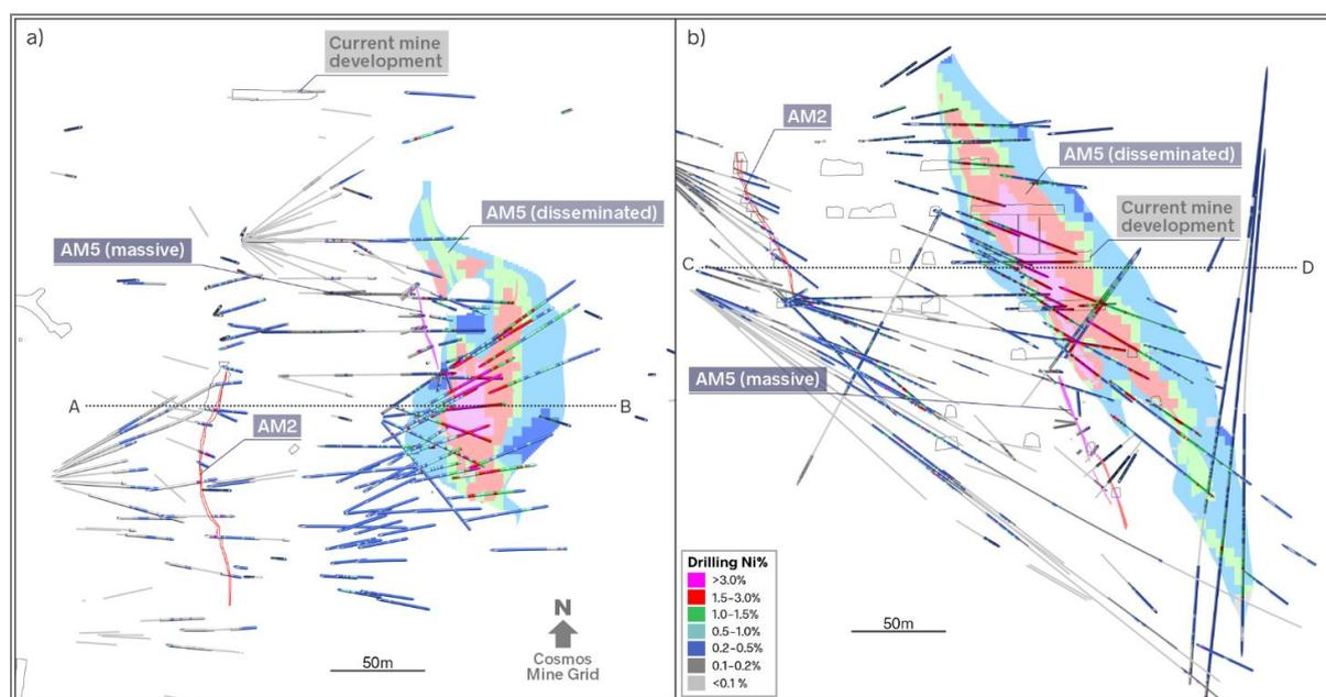
Notes: a) Plan view at level C to D denoted by the dotted line in the image to the right. b) Section view at northing A to B in denoted by the dotted line in the image to the left
