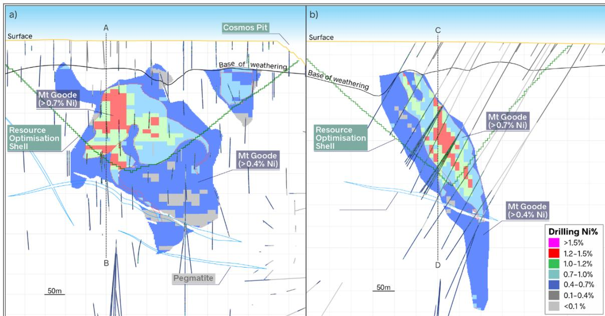
Notes: a) Long section looking west on the section line C to D denoted by the dotted line in the image to the right. b) Cross section looking north on the section A to B denoted by the dotted line on the image to the left.
