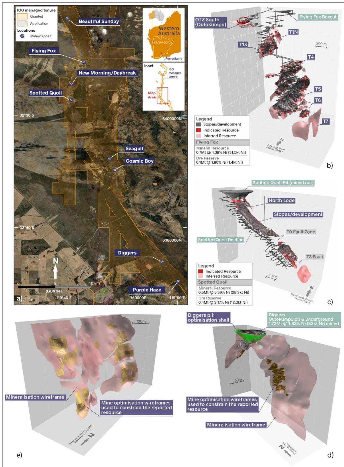
Notes: Clockwise from top left: a) Nickel deposits at Forrestania. b) Flying Fox mine. c) Spotted Quoll mine. d) Diggers mineralisation limits, FY23 RP3E MSO MRE reporting shapes, prior open pit, and FY23 RP3E pit optimisation shell. e) NMDB mineralisation limits and FY23 RP3E MSO MRE reporting shapes.
