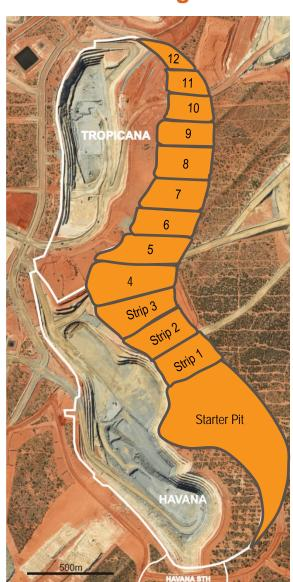
**Step 1: Mine starter pit - waste dumped ex-pit**
