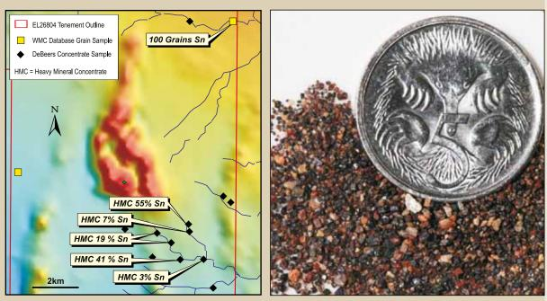
**Figure 24:** Birrindudu – (a) Tin Rich Heavy Mineral Concentrate Locations Over Aerial Magnetic Image (b) Photograph of Cassiterite-Rich Heavy Mineral Concentrates
