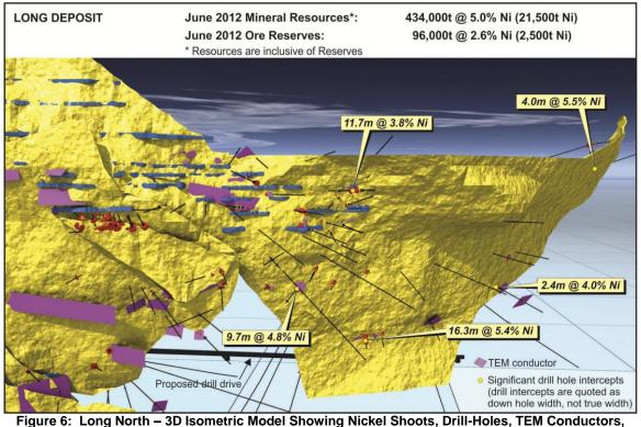
gure 6: Long North – 3D Isometric Model Showing Nickel Shoots, Drill-Holes, TEM Conductors Proposed Development and Significant Intercepts.
