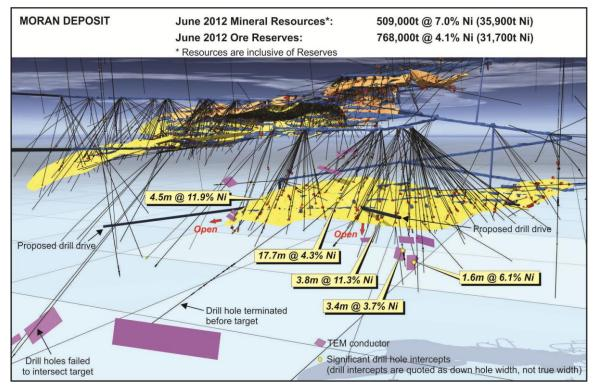
Figure 4: Moran - 3D Isometric Model Showing Nickel Shoot, Drill-Holes, TEM Conductors, Proposed Development and Significant Intercepts.
