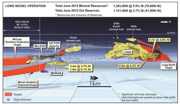
Figure 3: Long Nickel Mine – Longitudinal Projection Showing Target Areas, TEM Conductors and Significant Intercepts FY 12.
