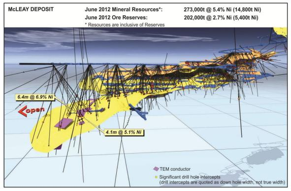
Figure 5: McLeay – 3D Isometric Model Showing Nickel Shoots, Drill-Holes and Development.
