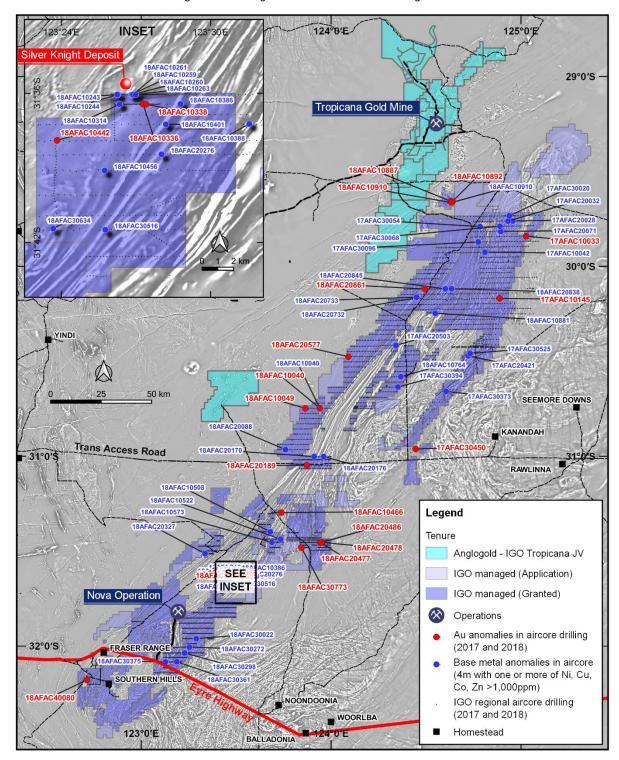
Fraser Range aircore drilling locations and anomalous drilling results to date
