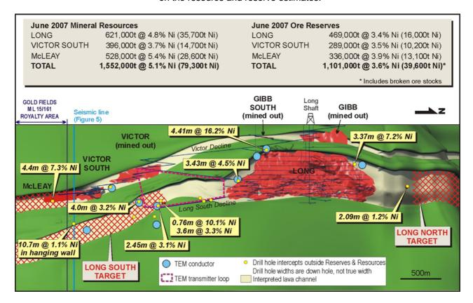
Figure 1: Long Nickel Mine – Longitudinal Projection Showing Lava Channels, Significant Intercepts Outside Current Resources and 2007/8 Exploration Targets
