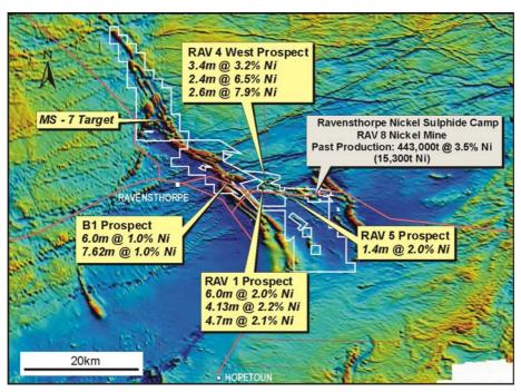
Figure 14: Ravensthorpe JV - Project Tenure Over Magnetic Image Showing Prospects and Significant Intercepts
