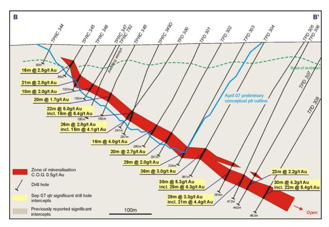
Figure 10: Tropicana JV - Havana Zone TPRC344 - TPD308 Cross-Section Showing Significant Drill Hole Results and the April 2007 Preliminary Conceptual Open-Pit Outline
