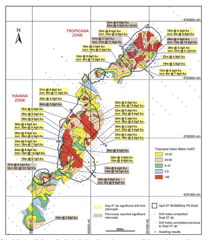
Figure 7: Tropicana JV - Prospect Plan Showing Significant Intercept Locations, g/t Au x Thickness (m) Contours, and Location of the Havana and Tropicana Zones
