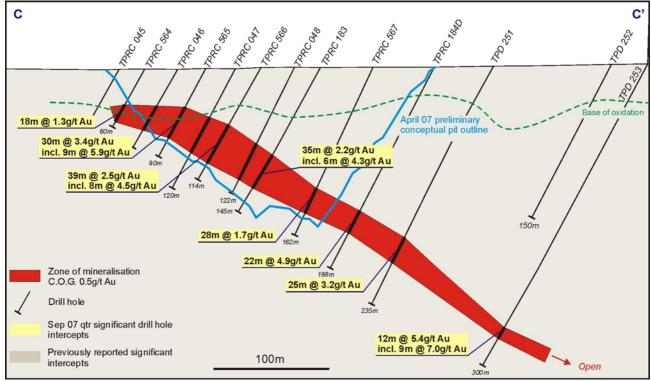
Figure 11: Tropicana JV - Tropicana Zone TPRC045 – TPD253 Cross-Section Showing Significant Drill Hole Results and the April 2007 Preliminary Conceptual Open-Pit Outline
