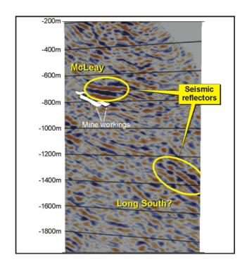
Figure 5: McLeay and Long South Seismic Section Showing Reflector Anomalies Possibly Associated with Nickel Sulphide
