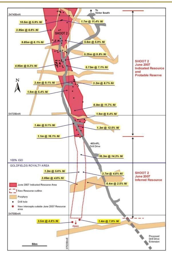
Figure 3: McLeay - Shoot 2 Plan Showing Significant Intercepts, Resource Boundaries and Drill Drive Location.
