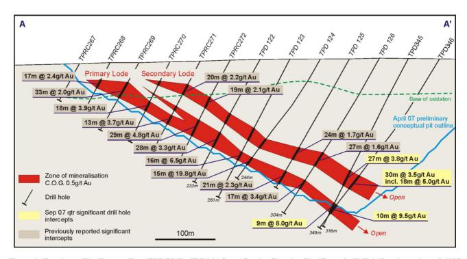
Figure 9: Tropicana JV - Havana Zone TPRC267 - TPD346 Cross-Section Showing Significant Drill Hole Results and April 2007 Preliminary Conceptual Open-Pit Outline
