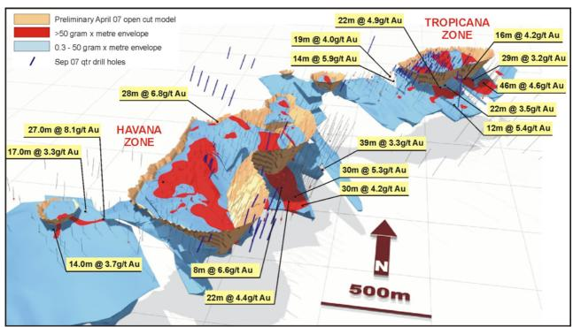
Figure 8: Tropicana JV – Isometric Model Showing 0.3g/t Au Mineralised Envelope, g/t Au x Thickness (m) Contours Within, and Significant Intercepts Outside, the April 2007 Preliminary Conceptual Open-Pit Outline
