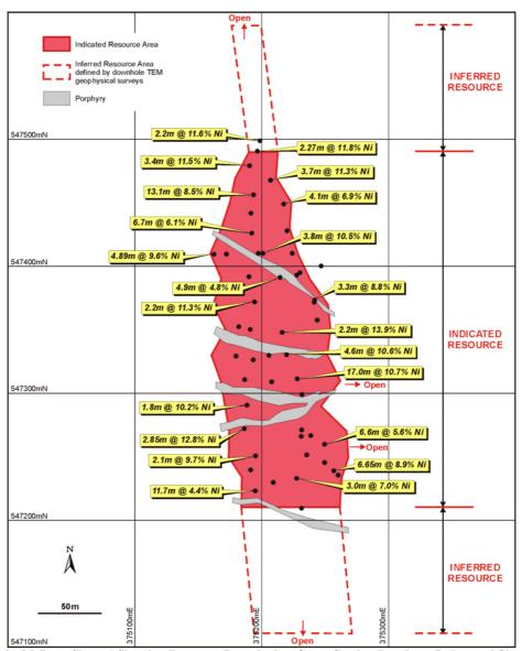
Figure 2: McLeay Shoot 1 Showing Resource Boundaries, Cross Cutting Porphyry Dykes and Significant Intercepts
