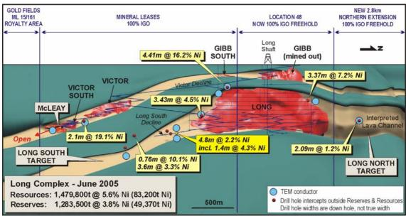
Figure 1: Long Nickel Mine – Longitudinal Projections Showing the Location of McLeay Proximal to Existing Victor South Decline Development
