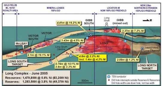
Figure 1: Long Nickel Project - Longitudinal Projection
