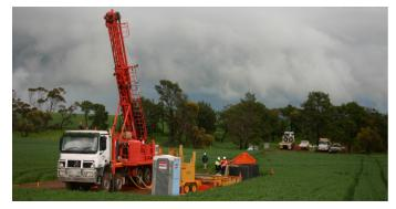
Figure 3: Diamond rig drilling on cropped land
