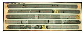
Figure 2: Diamond drill core laid out in core tray
