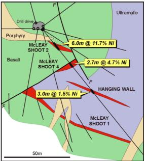
Figure 3: McLeay Shoot 2 - 547,210mN Cross-Section Showing Resource Boundaries, Cross-Cutting Porphyry Dykes, Drill-holes, Significant Intercepts and the Location of the 460 Development Drill Drive
