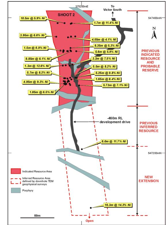
Figure 2: McLeay Shoot 2 Plan Showing Resource Boundaries, Cross-Cutting Porphyry Dykes, Significant Intercepts and the Location of the 460 Development Drive
