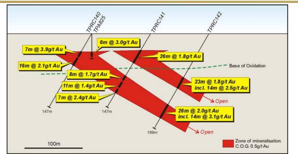
Figure 15: Tropicana JV – Havana Zone TPRC140-TPRC142 Cross-Section Showing Significant Drill Hole Results
