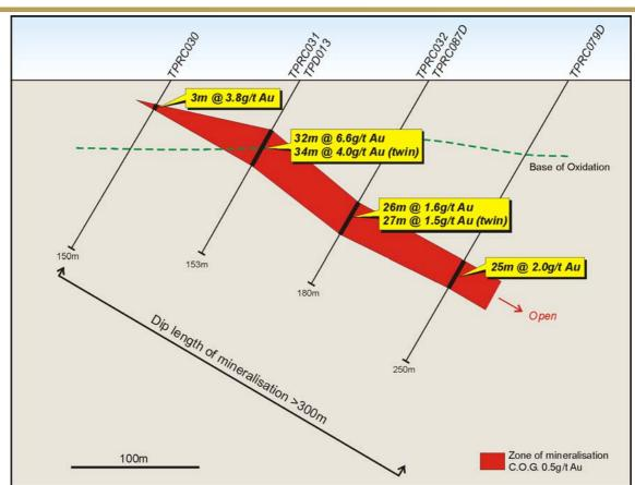
Figure 13: Tropicana JV – Tropicana Zone TPRC019-TPRC021D Cross-Section Showing Significant Drill Hole Results
