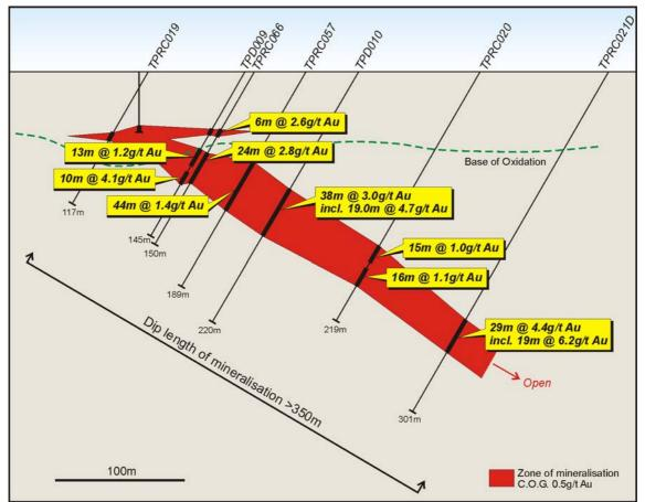
Figure 14: Tropicana JV – Tropicana Zone TPRC030-TPRC079D Cross-Section Showing Significant Drill Hole Results
