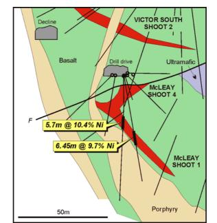
Figure 1: McLeay Shoot 1 - 547,450mN Cross-Section Showing Resource Boundaries, Cross-Cutting Porphyry Dykes, Drill Holes and Significant Intercepts and the Location of the 460 Development Drill Drive
