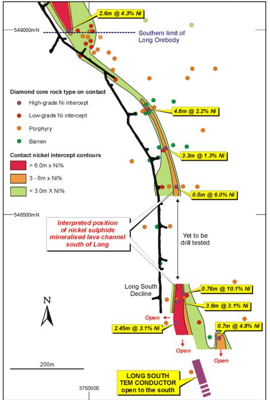
Figure 4: Long South Exploration Decline Plan Showing Significant Drill-Hole Hits and Nickel % x thickness (m) Mineralisation Envelopes and TEM Conductor, Open to the South
