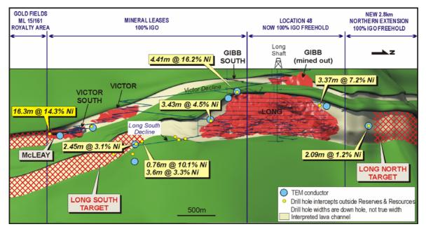
Figure 5: Long Mine Complex Longitudinal Projection Showing the Long South and Long North Target Access and Significant Intercepts Outside Current Reserves and Resources
