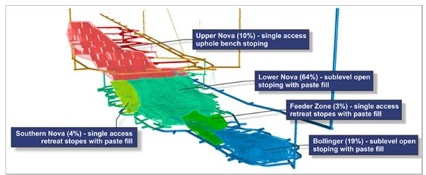
Figure 2: Generalised stoping areas for the Nova Project.
