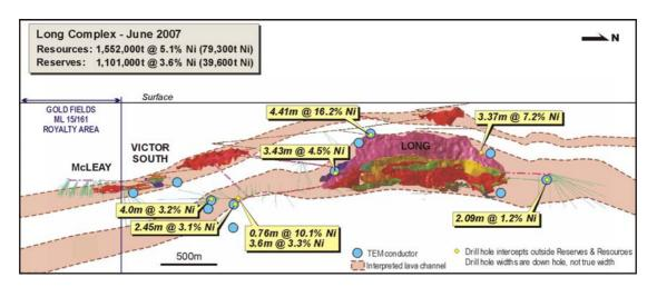
Figure 3: Long Nickel Mine – Longitudinal Projection Showing Significant Intercepts Outside Current Resources and Reserves
