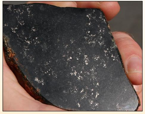
Figure 1. Quick Shears outcropping nickel-copper sulphide hand specimen
