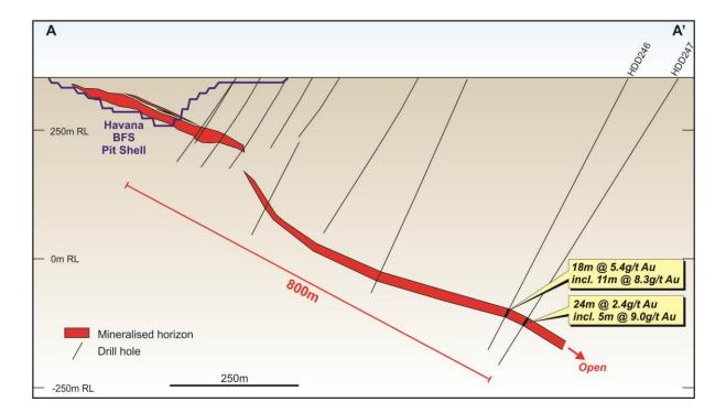
Figure 2: Cross Section A-A' Illustrating the New Gold Intercepts Down Plunge from the Havana BFS Pit Outline.
