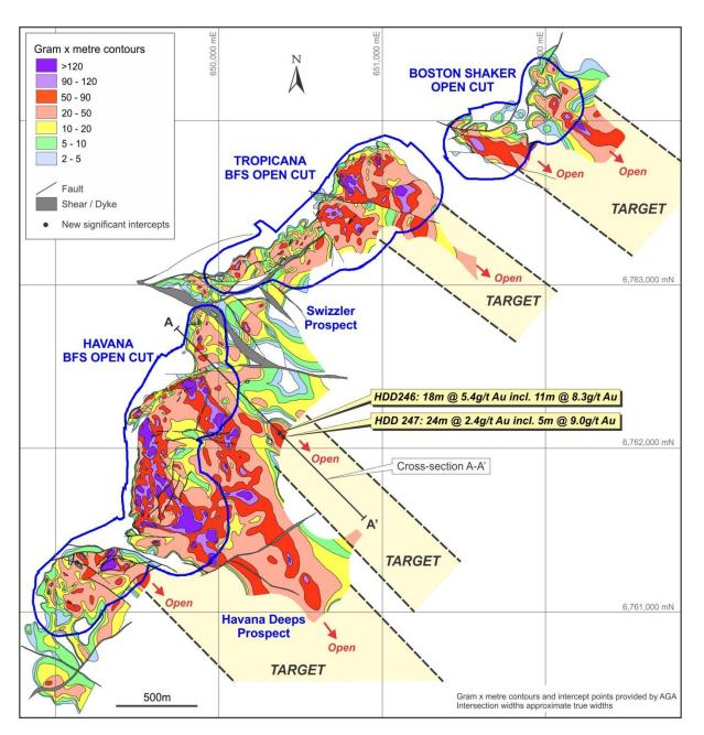
Figure 1: Proposed open pit positions with Grade (Au) x Thickness Contours and New Gold Intercepts down plunge of Havana North.
