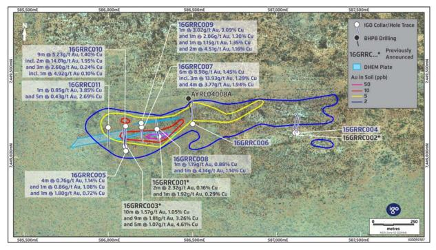
Figure 3: Grapple Prospect showing the location of the eleven drill holes and the main Au and Cu mineralized zones.
