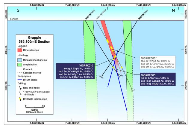
Figure 4: Grapple Prospect 586100E cross section.
