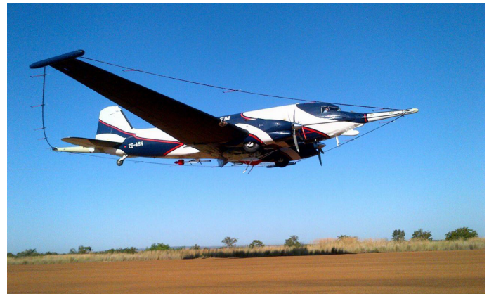
Figure 2: Example of fixed wing SPECTREM plane landing after completing an electromagnetic survey
