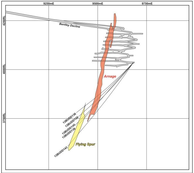
Figure 1. Composite cross-section of Bentley ore body showing position of Flying Spur Lens relative to Arnage and recently completed underground drill holes and mine development.
