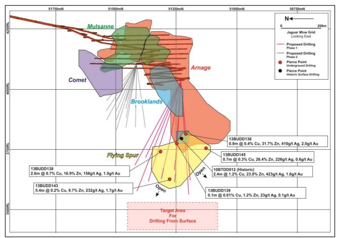
Figure 2: Long Section of Bentley ore body showing location of Flying Spur in relation to other lenses, intercepts and point from the recently completed underground drill program and planned phase one (pink) and phase two (blue) follow-up drilling
