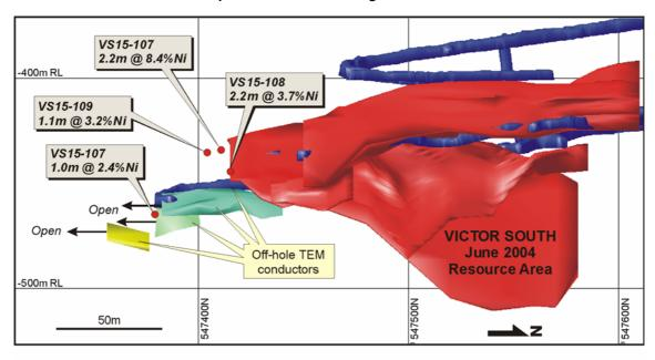
Figure 2: Victor South model showing off-hole MagTEM conductors and new intercepts south of the current resource area
