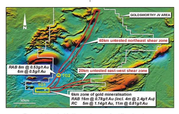
Figure 4: Goldsworthy Joint Venture – Aeromagnetics, drill results and targets
