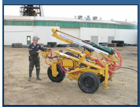
Compressed air blast hole rig
