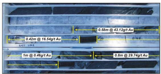
Figure 2: Francis Furness Diamond Drill Hole FFD4 Drill Core – East Lode Intersection 2.8m @ 20.07 g/t Au
