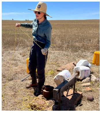
Figure 2: Using a hand bailer to collect water from a bore
