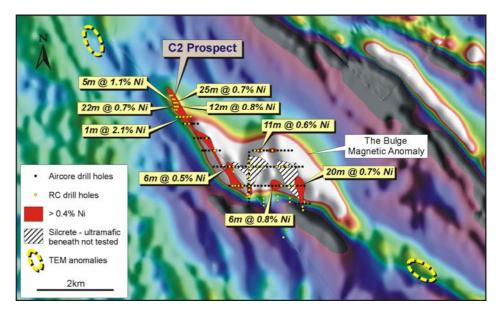
Figure 11: Duketon JV – Bulge C2 Prospect Magnetic Anomaly, Significant RC and AC Drill Results, > 0.4% Ni Anomalism and TEM Anomalies Over Aeromagnetic Image
