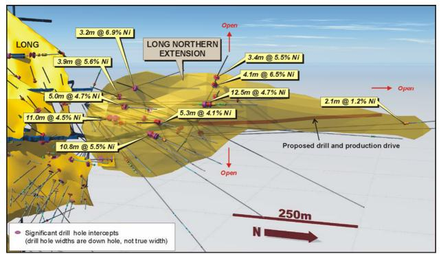
Figure 3: Long North 07 Shoot - Longitudinal Projection Showing Workings, Significant Intersections and Resource Boundary
