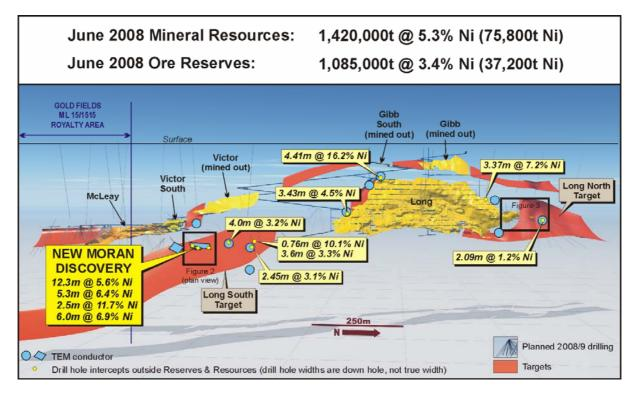
Figure 1: Long Nickel Mine - Longitudinal Projection Showing Target Areas, TEM Conductors, Significant Intercepts Outside Current Resources and Reserves, Proposed 2008/9 Exploration in Light Blue and Figures 2 and 3 Locations
