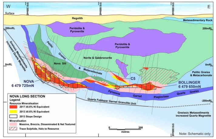
Figure 1: Schematic Long Section of the Nova-Bollinger – Looking North
