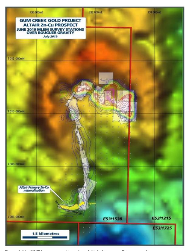
Figure 8-23: MLEM survey results and modelled plates over Bouger gravity
