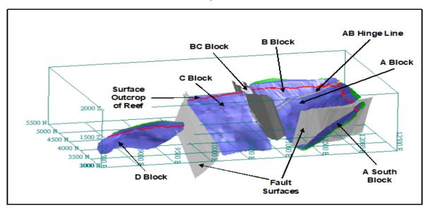
Figure 5-1: Wireframes showing the Panton 101 and 201 reef system
