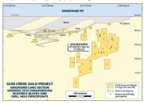
Figure 8-8: Section showing mineralisation and previous workings at the Kingfisher deposit Source: Horizon Prospectus (October 2016)
