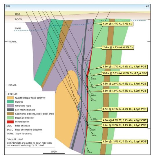
Figure 5: Rosie cross-section with mineralisation
