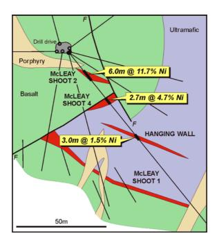
Figure 1: McLeay Deposit - 547,210mN Cross-section Showing MDU-117 Intercept
