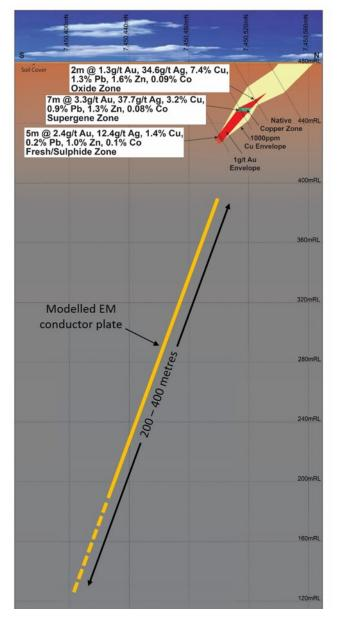
Figure 2: Cross-section on 588,300mE showing modelled plate and air-core drill hole intercepts
