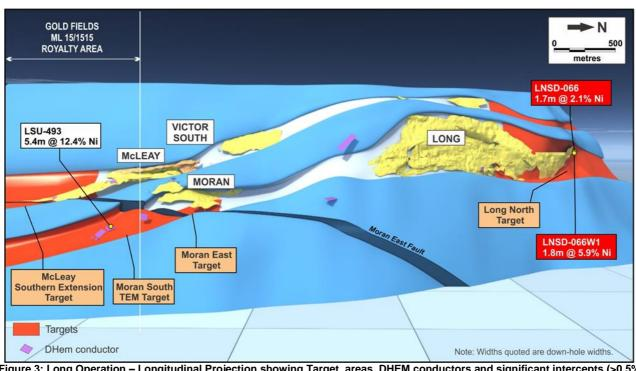
Figure 3: Long Operation – Longitudinal Projection showing Target areas, DHEM conductors and significant intercepts (>0.5% Ni)- (see ASX release dated 10 December 2014 for further detail on the Moran South drill result).
