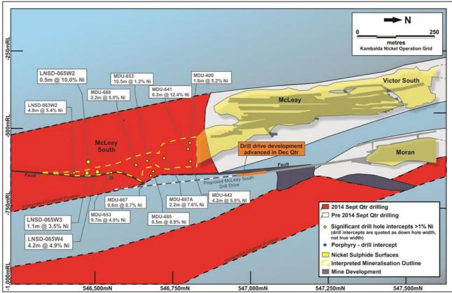
Figure 4: Long Operation – Longitudinal Projection showing McLeay South Target areas, TEM conductors, significant intercepts (>0.5% Ni) and McLeay South Drill Drive advance.
