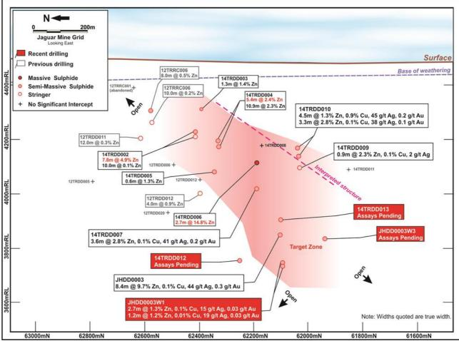
Figure 6 : Jaguar Operation Regional Exploration - Triumph Long Section. (see ASX release dated 22 September 2014) Note: Previous Triumph Long Sections disclosure to ASX had North pointing to right of the figure.
