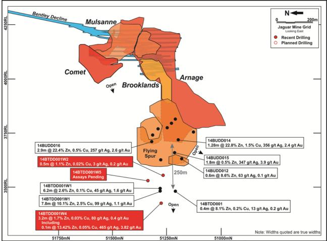
Figure 5: Jaguar Operation: Bentley Composite Long Section showing location of Flying Spur and Bentley Deeps drill holes. Down hole widths are true widths. Note: North is to the left in the diagram. See ASX release dated 22 September 2014
